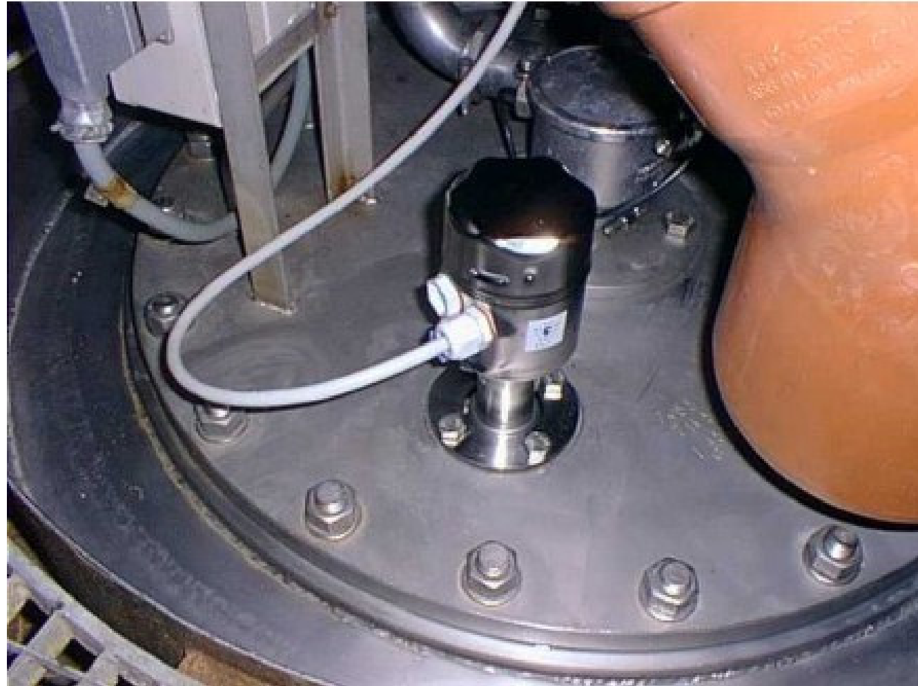
CO 2 - head pressure measurement at the fermentation tank in the brewery with Deltapilot S DRD-flange
