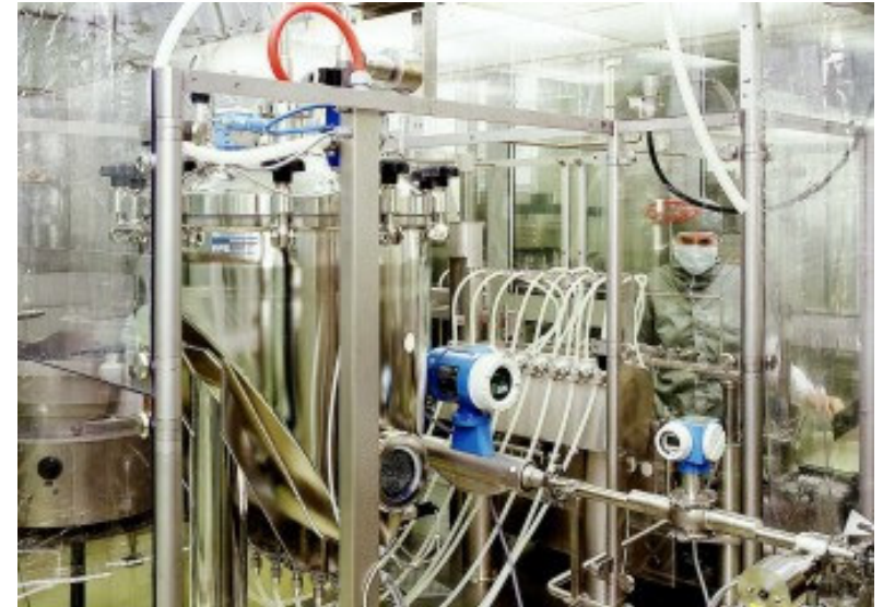
Pressure measurement in a pharmaceutical unit with Cerabar S PMC731, Varivent-housing
